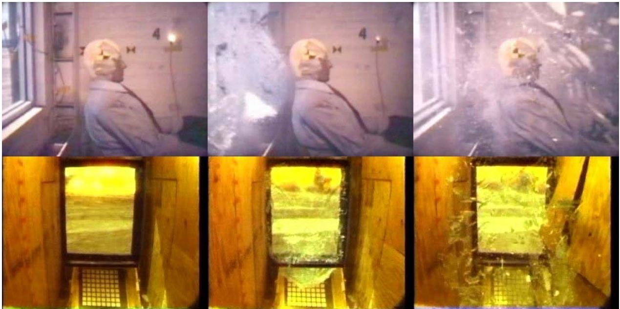
Fig. 1 Burst of a single window after an explosion (source: US Army Corps of Engineers)
